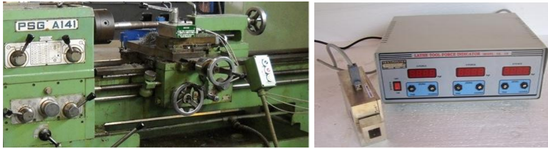
Fig. 2 (a) Experimental setup; (b) Lathe tool force indicator.
